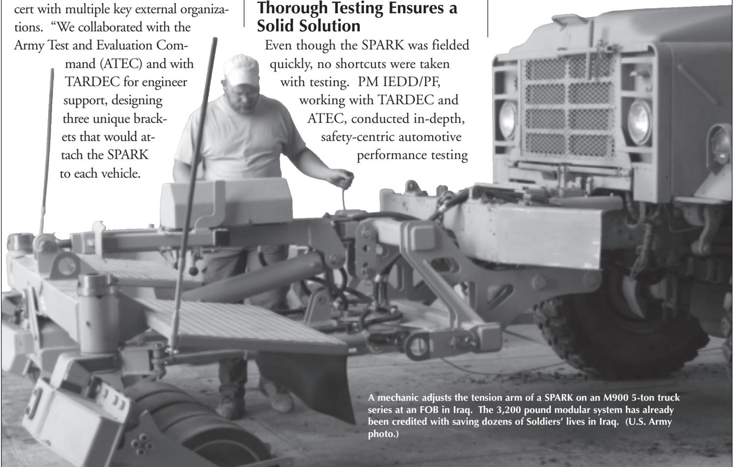
A mechanic adjusts the tension arm of a SPARK on an M900 5-ton truck series at an FOB in Iraq. The 3,200 pound modular system has already been credited with saving dozens of Soldiers' lives in Iraq. (U.S. Army photo.)
