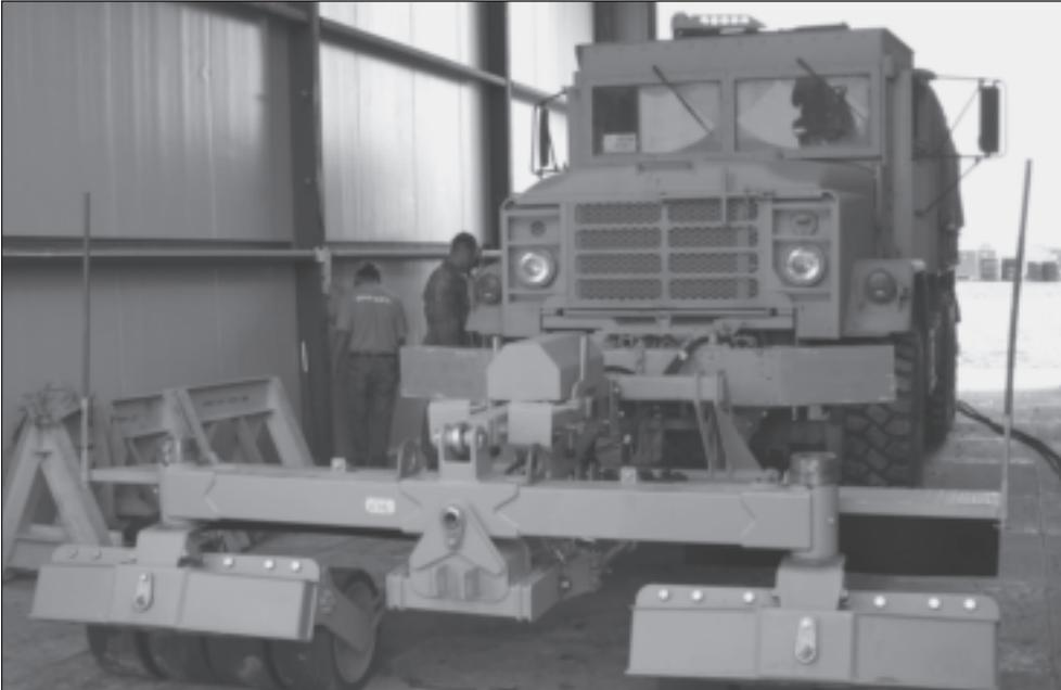
Here, technicians finish outfitting an M900 5-ton truck series with SPARK at an FOB in Iraq. The rollers are designed to defeat pressure-sensitive triggered IEDs by forcing the blast down and away from the vehicle. (U.S. Army photo.)
